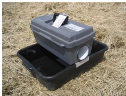
Gravid Trap Nutrient rich water attracts female mosquitoes that are looking to lay eggs
